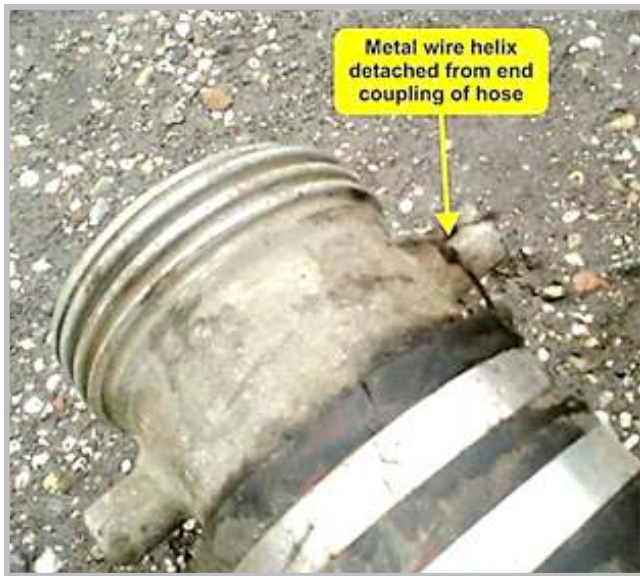
Figure 3 . An isolated coupling caused by a broken wire helix.
